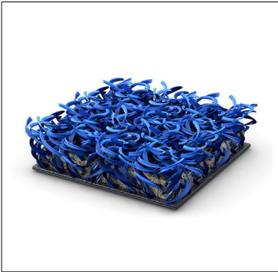
Latest generation artificial turf, manufactured with linear tufting process. It has a gauge of 3/16" with 22 tufts/dm, resulting in 46.200 tufts/m<sup>2</sup>. The Premier Supercourt X3 available in different colors, yarns have a height of 10 mm and 8.200 dtex.
