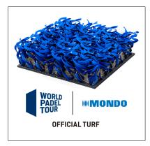
Latest generation artificial turf, manufactured with linear tufting process. It has a gauge of 3/16" with 22 tufts/dm, resulting in 46.200 tufts/m<sup>2</sup>. The Supercourt XN available in different colors yarns have a height of 10 mm and 8.610 dtex.
