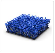
State-of-the-art artificial grass system, manufactured using an in-line tufting system of a 3/16" gauge size with 17 point/dm, resulting in 35,700 point/m<sup>2</sup> with SHOT XN blue grass filaments of 10 mm height and 9.000 dtex.
